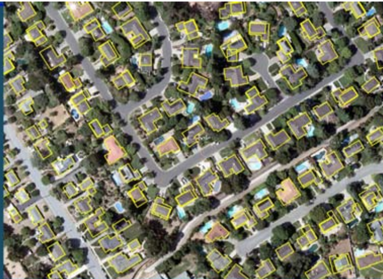
Building polygons are drawn manually. Most polygons are orthogonal, they can be partitioned into rectangles.
