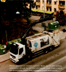
Latest addition to the Resta fleet is this of large four-axle Volvo chassis - with 'indoor' rear bogie - fitted with NTM vacuum waste collection system, and capable of sucking over 3-tonnes per hour through underground pipes.
