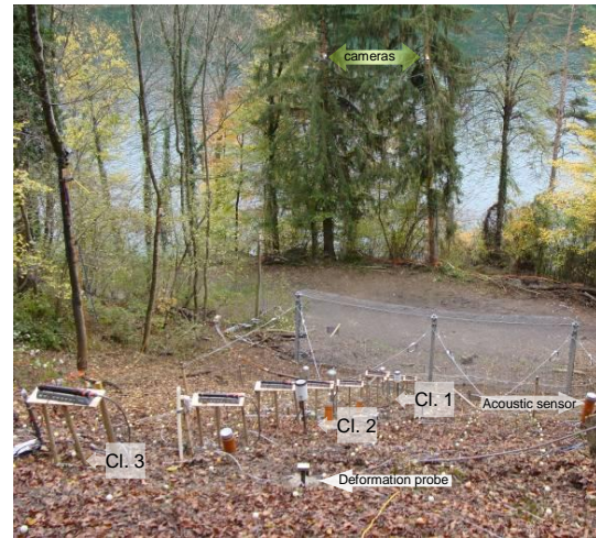
Location of instrumentation clusters (Cl. 1 – 3), the sprinklers and the photogrammetry cameras.
