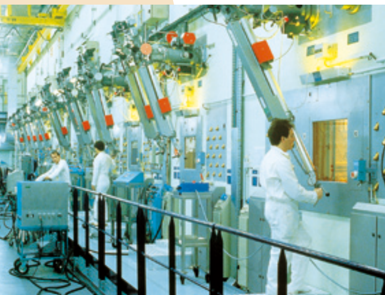
Remote handling in dismantling cell.
