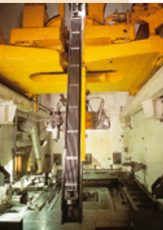
Tilting crane: feeder bridge in shearing facility.
