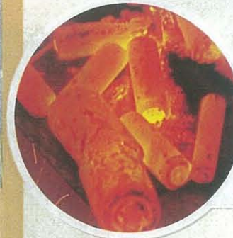
Batteries heated in the furnace
