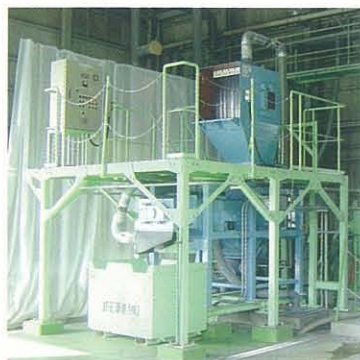
Crushing facility Processing capacity: 1,500 tons/month
