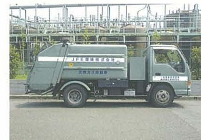
Yokohama City 2 ton compacting refuse collector
