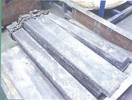
Cadmium abstracted from Ni-Cd Battery at Bell Vacuum Electric Furnace
