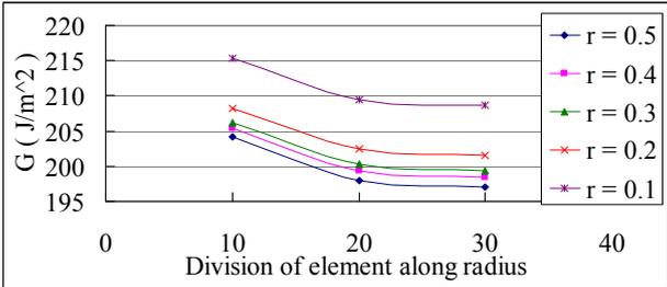
Fig4 Convergence test of double cantilever beam model
