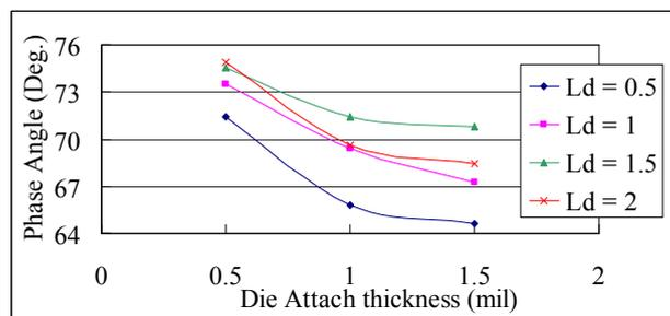
Fig. 19 Effect of Die Attach Thickness on Mode Mixity
