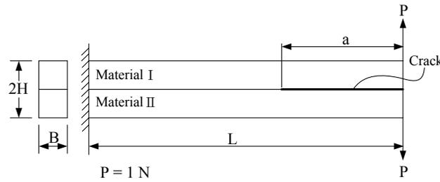
Fig1 Double cantilever beam model
