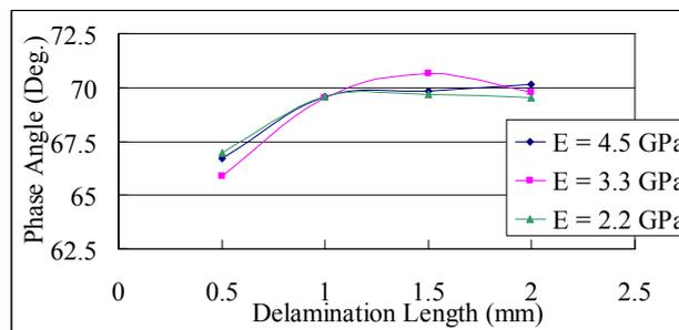
Fig. 17 Effect of Young's Modulus of Die Attach on Mode Mixity (CTE = 131.3 ppm/°C)
