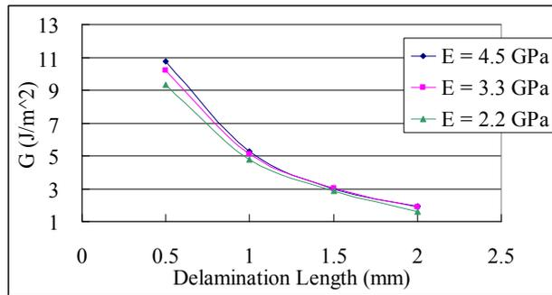
Fig. 7 Effect of Young's Modulus of Die Attach on Delamination (CTE = 131.3 ppm/°C)
