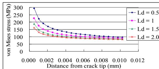
Fig. 12 Effect of Delamination Length on Stress Distribution along Crack Tip (D/A thick. = 0.5 mil)
