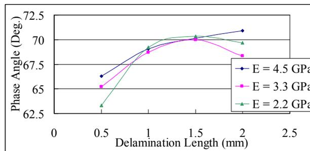
Fig. 18 Effect of Young's Modulus of Die Attach on Mode Mixity (CTE = 89.7 ppm/°C)
