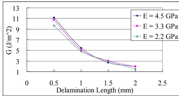
Fig. 6 Effect of Young's Modulus of Die Attach on Delamination (CTE = 172.8 ppm/°C)
