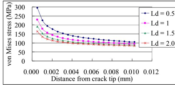
Fig. 13 Effect of Delamination Length on Stress Distribution along Crack Tip (D/A thich. = 1 mil)
