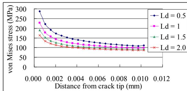
Fig. 14 Effect of Delamination Length on Stress Distribution along Crack Tip (D/A thich. = 1.5 mil)
