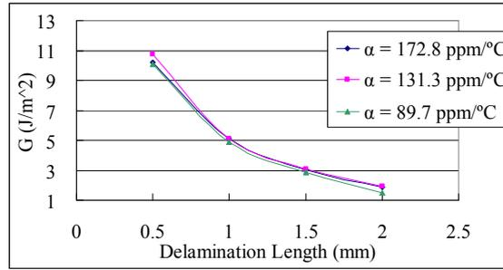
Fig. 10 Effect of CTE of Die Attach on Delamination (E = 3.3 GPa)
