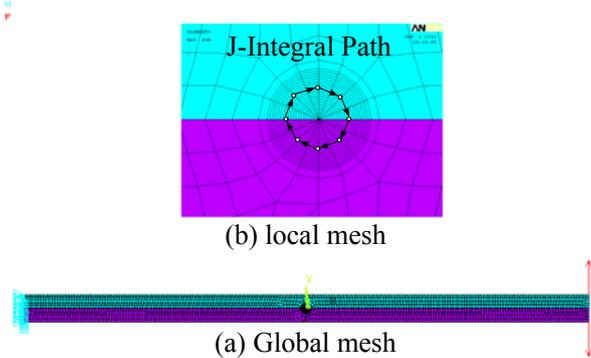
Fig. 3 Finite element model of double cantilever beam
