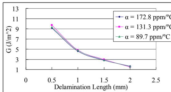
Fig. 11 Effect of CTE of Die Attach on Delamination (E = 2.2 GPa)
