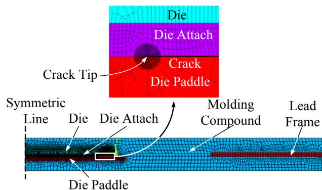
Fig. 5 Finite element mesh of TSOP with crack
