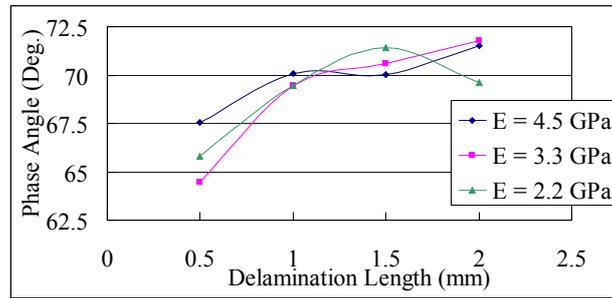
Fig. 16 Effect of Young's Modulus of Die Attach on Mode Mixity (CTE = 172.8 ppm/°C)
