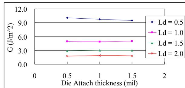
Fig. 15 Effect of Die Attach Thickness on Delamination
