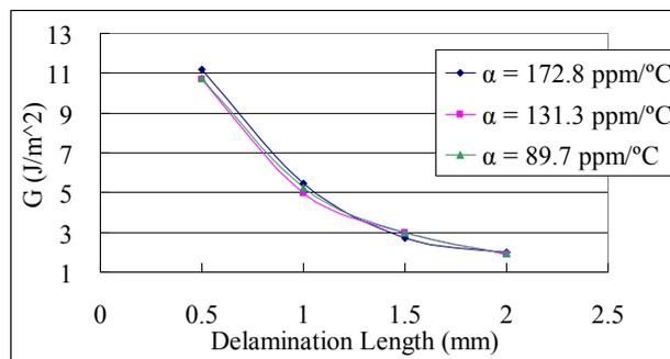
Fig. 9 Effect of CTE of Die Attach on Delamination (E = 4.5 GPa)
