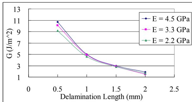
Fig. 8 Effect of Young's Modulus of Die Attach on Delamination (CTE = 89.7 ppm/°C)
