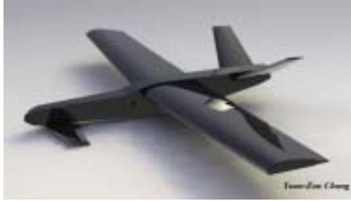
Figure 12. Devil Bat. As the first mini uninhabited aerial vehicle with three-surface configuration designed by the adapted airplane sizing method, Devil Bat has the canard, V-tail, high wing, and the pusher-type engine. (Copied from Yuan-Zun Chang's final report with his permission.)
