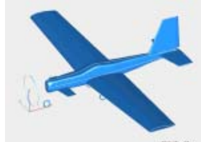
Figure 13. Monk Vulture (Proposed Configuration). To improve directional stability of TYLL-L and to carry more payloads, Monk Vulture has a similar shape, but with a canard, compared with TYLL-L. This mini UAV is a traction-type engine propeller-driven air vehicle.
