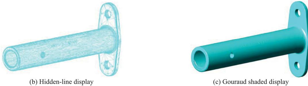
Figure 1. Triangular mesh model of a cable support
