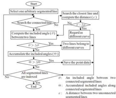
Figure 12. Procedure of extracting reduced contour points
