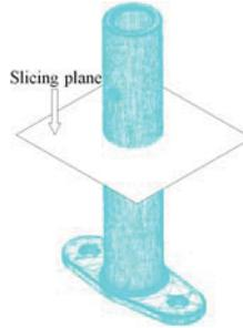
Figure 9. Slice cutting through the STL model
