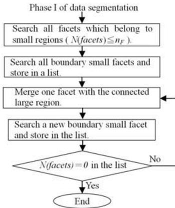
Figure 6. Procedure of mesh redistribution
