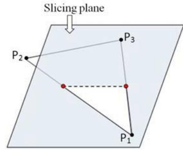
Figure 10. Two intersection points on the slicing
