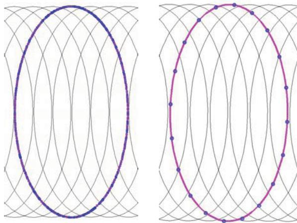
(a) Contour of segmented lines (b) Contour of NURBS
