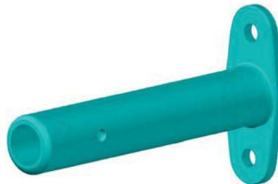
(b) Reconstructed solid model for the cable support
