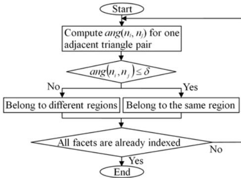
Figure 2. Procedure of mesh segmentation
