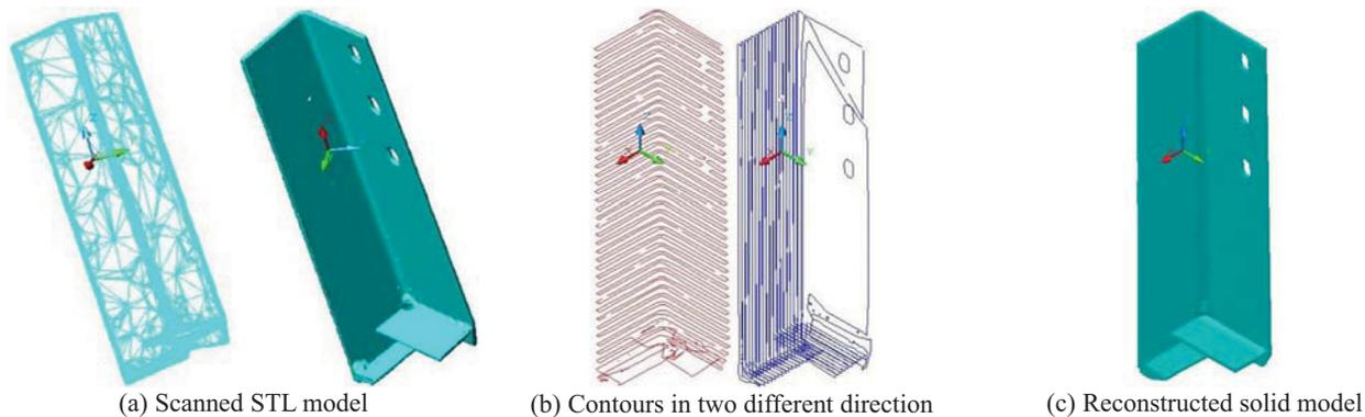
Figure 16. Solid model reconstruction of the angle plate
