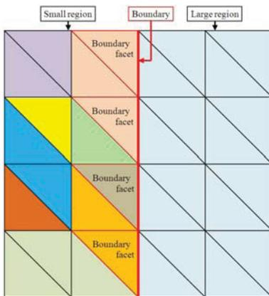
Figure 5. Schematic of small boundary region facets
