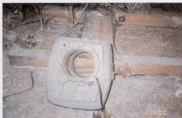
圖 7 : The teletherapy head with the missing source drawer assembly was found after the accident
