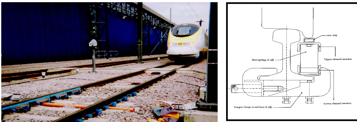
圖39&40. Roundchex車輪狀態監視( From DeltaRail)
