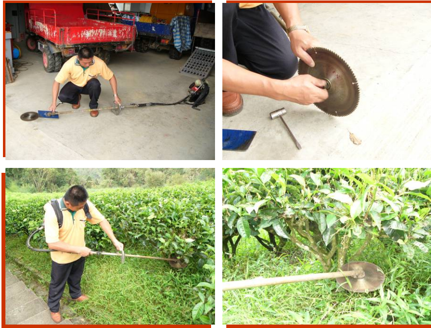
Fig 11. The pruning equipment modified from a lawn mower.
