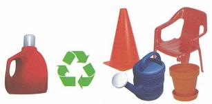
High density plastics (#2) such as detergent bottles are sorted and ground into flakes. These flakes can form new materials such as plastic patio furniture, watering cans, flower pots, traffic cones, or drainage pipes.
