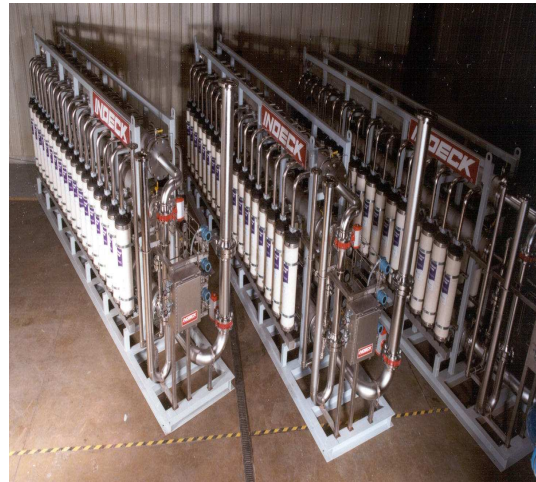
3 UF Racks Produce 2.1 MGD Product Water for RO Feed
