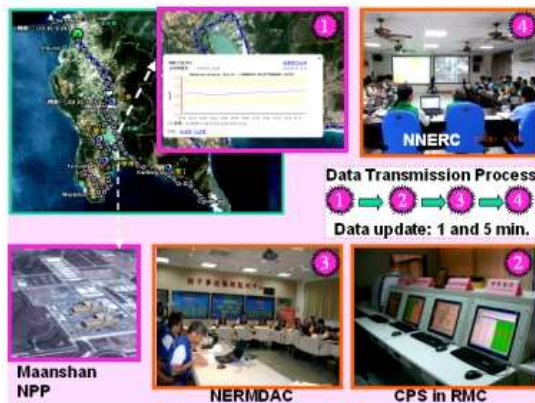
Fig. 5. The EGMN data transmission process was divided into four steps during the 2008 nuclear emergency exercise. The data were transmitted to CPS in RMC in real time, and integrated with the geography information in automatic.
