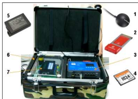
Fig. 2: The structure of a mobile device, it mainly includes (1) a GPS as positioning receiver; (2) a Wireless communication interface card; (3) a compact computer for the data processing analysis; (4) a Memory card; (5) a Lithium battery; (6) a detector probe as Geiger-Mueller tube, ionization chamber, or scintillation instruments; and (7) a Micro-processor module with a screen monitor.
