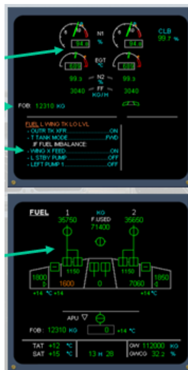
圖 3.4-3 ECAM DISPLAY (UPPER: ENGINE and Warning Display, Down: System Display)
