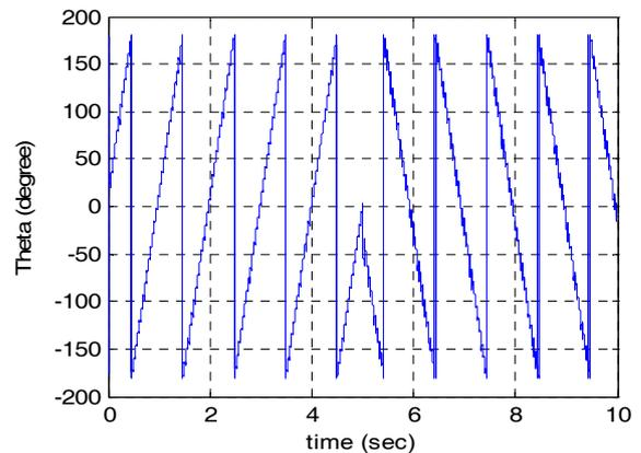
Figure 7(c). The simulation result for flux position response ( $\theta$ ).
