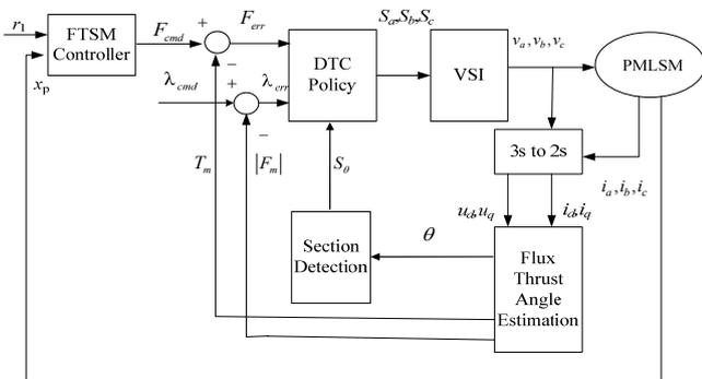
Figure 6. The block diagram of a simulated PMLSM control system.
