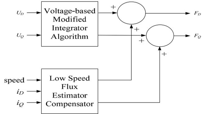
Figure 4. A flux estimator block diagram with flux compensator.
