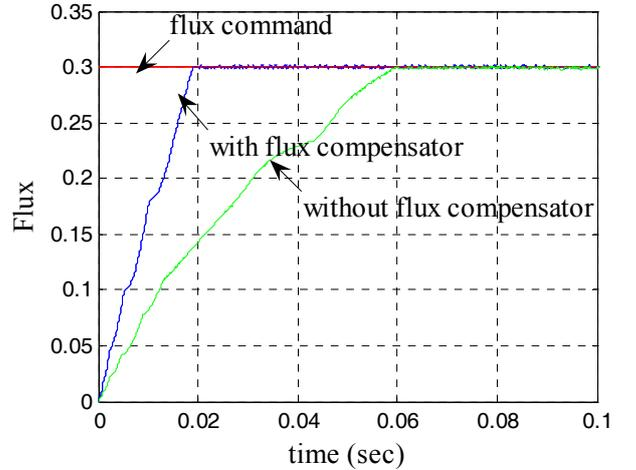
Figure 5. The flux linkage response with/without flux compensator.
