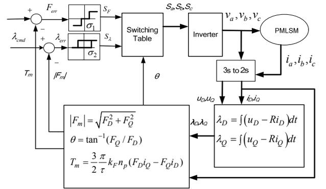
Figure 1. A PMLSM control block diagram using DTC policy.
