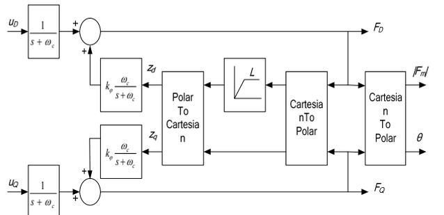
Figure 2. A voltage-base modified integrator block diagram.
