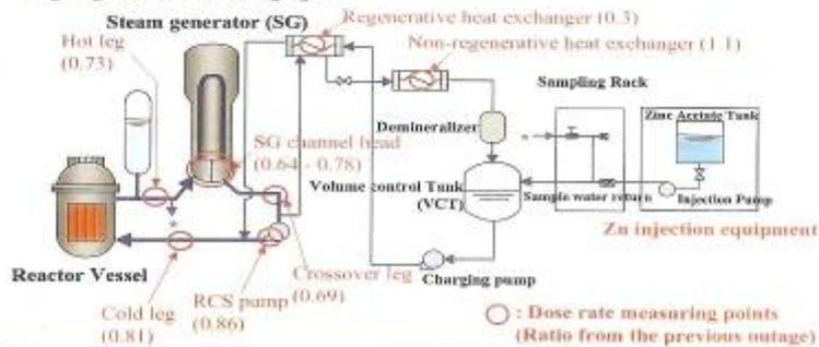
The zinc injection reduced the dose rate of primary equipment and pipes to 70-80 % than that of previous outage. This effect of dose reduction is higher than expectation based on the foregoing plants. However non-regenerative heat exchanger had no effect of zinc injection.
