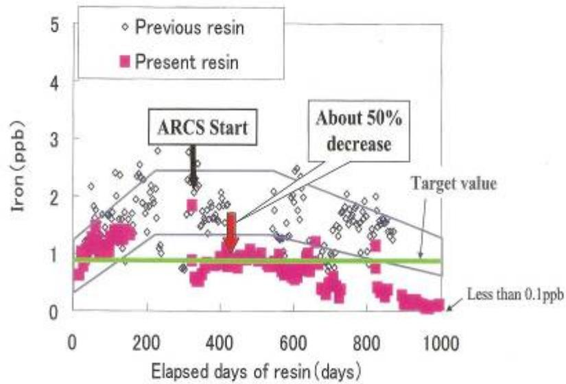
Feed water iron concentration after ARCS became less than half as high as that before ARCS.
