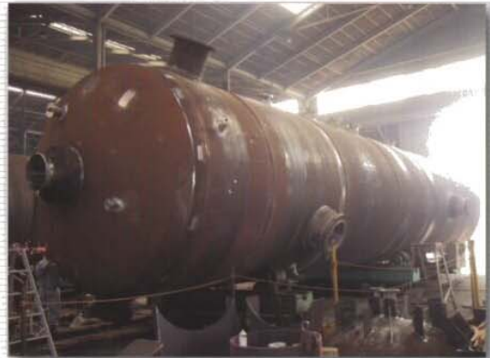
〈Pressure Vessel for Gas Clean-up〉
