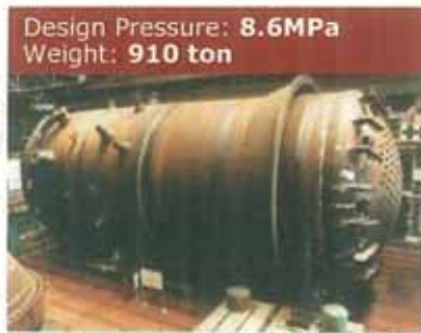
Reactor Pressure Vessel
