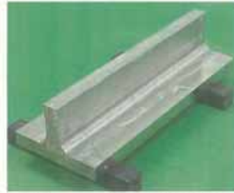
H9 weld mockup with SCC cracks
