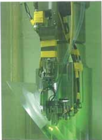
Laser Peening (Reactor Bottom Peening Device)
