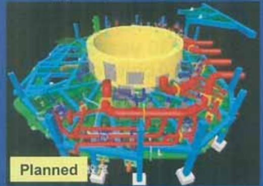
RCCV Upper Drywell Module (650 ton)
