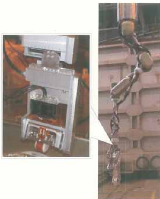
ECT scanner for CRD stub weld
