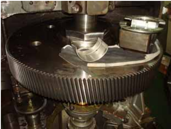
Gear for turbine of cargo pump
