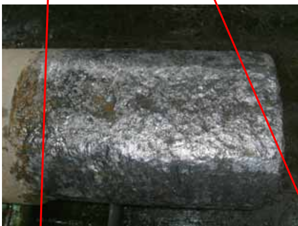
Heavy corrosion of connect end for coupling
