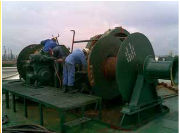
Windlass dismantled shaft with wire drum
