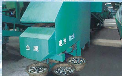
金屬、電池、打火機自動分選系統 Automatic Sorting System for Metals, Batteries and Lighters
