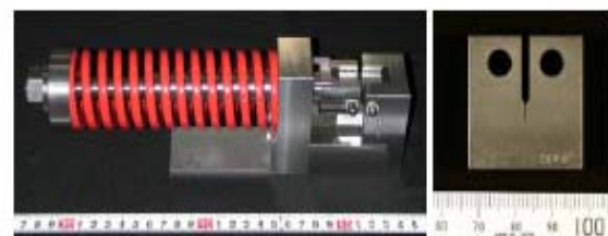
Fig.22. Crack Growth Test
