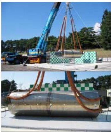
Fig. 9. Horizontal Drop Test
