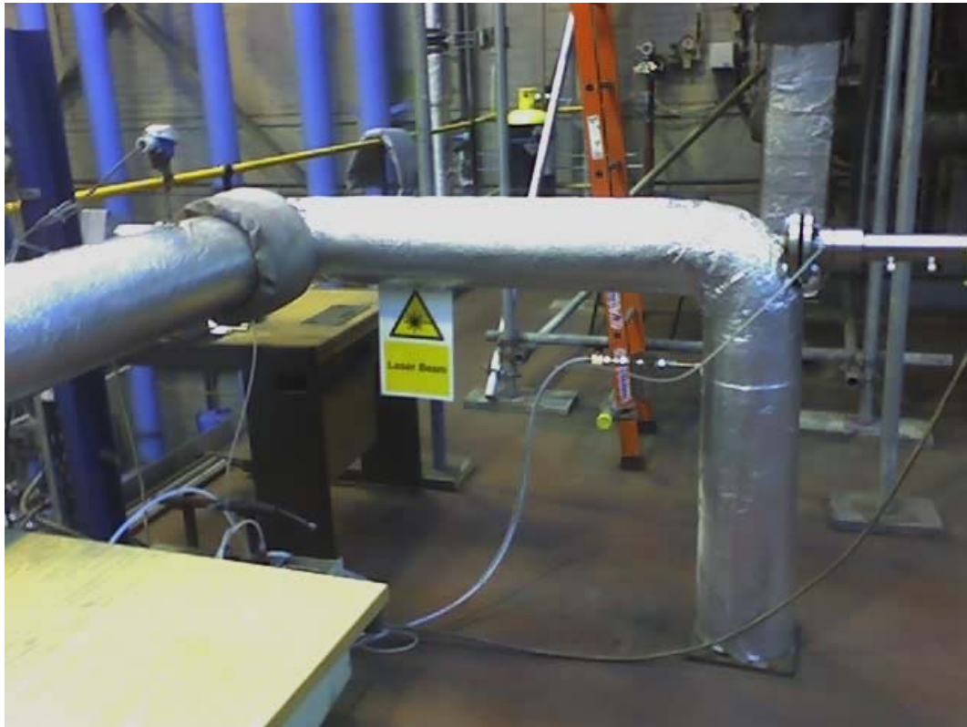
圖2.1.3-7 排放測試段(Emission testing section)
