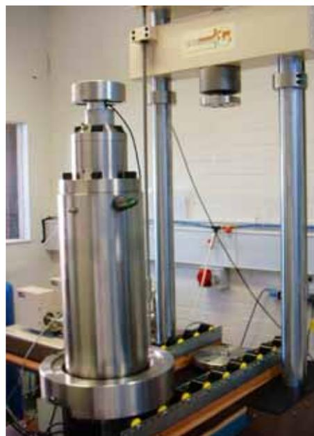
Figure 3.18 Fitting the triaxial cell into the loading frame
