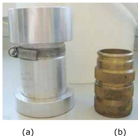
Figure 3.3 Moulds: (a) The mould of 5cm in diameter and 10 cm in height. (b) The mould of 3.8cm in diameter and 7.6cm in height.
