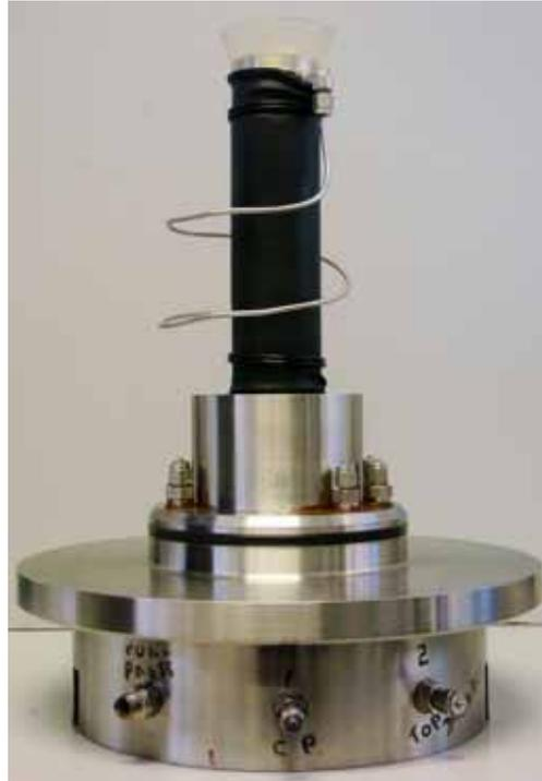
Figure 3.15 Prepared cemented specimen.
