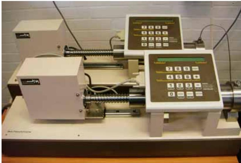
Figure 3.12 Advanced Digital Pressure/Volume Controller
