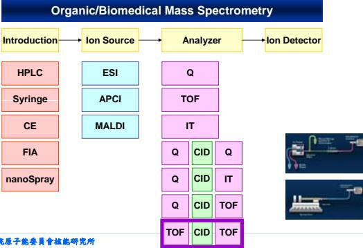
Introduction → Ion Source → Analyzer → Ion Detector
