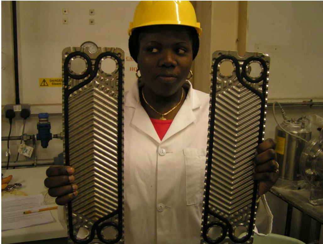
Fig. 2: The two different kinds of the plates which compose the exchanger alternately.
