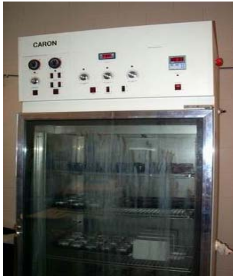
Environment Chamber – Damp Heat Badger Meter USA
