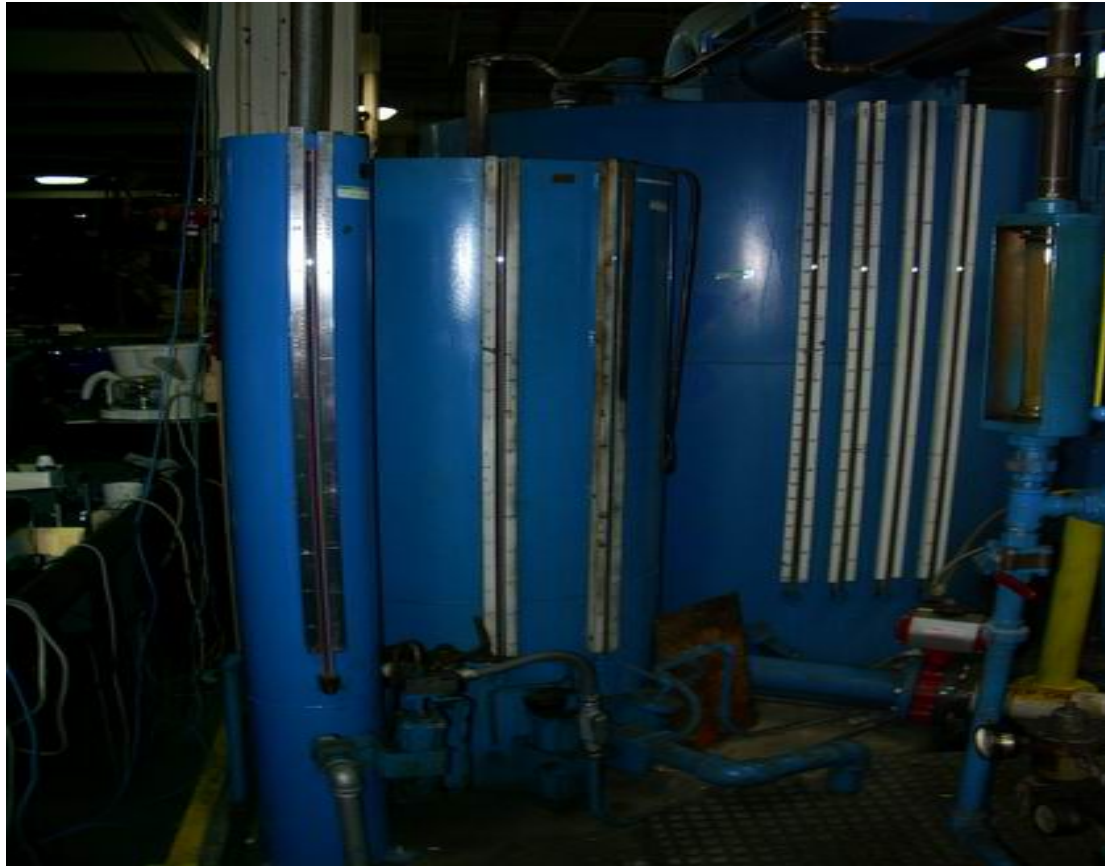
Different size tanks for various test quantities Badger Meter USA
