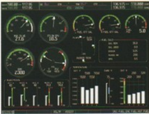
A comprehensive full-page display of engine, fuel and systems data can be accessed and monitored on the G900X MFD.
