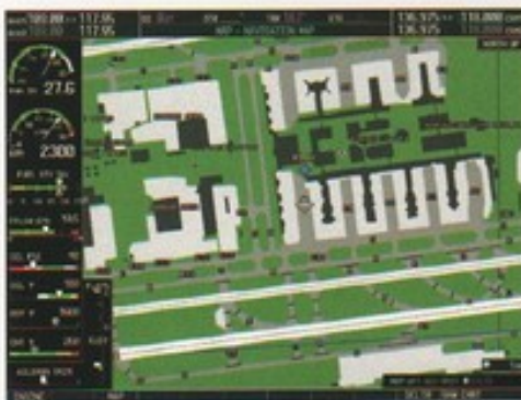
Built-in Garmin SafeTaxi™ airport diagrams in the G900X basemap help pilots identify runways, taxiways, hangars and aircraft location on over 680 U.S. airports.
