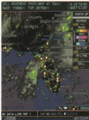
Weather datalink capability, via XM Satellite Radio and its XM WX Satellite Weather service, can provide the G600 with color NDWRAD, METARs, TAFs, lightning, and other U.S. data display.
