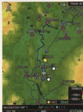
Traffic can be displayed on the moving map (as depicted), or on a stand-alone traffic page.
