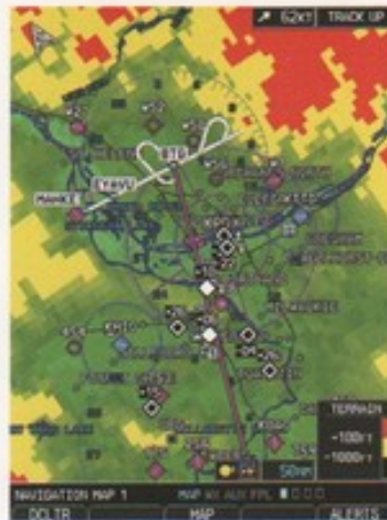
With its built-in elevation database, the G600 system provides an extra margin of safety in recognizing terrain/obstacle conflict situations.
