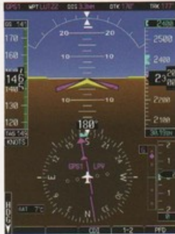
The pilot's Primary Flight Display (or PFD) seamlessly integrates all situational information regarding the aircraft's attitude, altitude, speed, heading, vertical rate, and flight progress.
