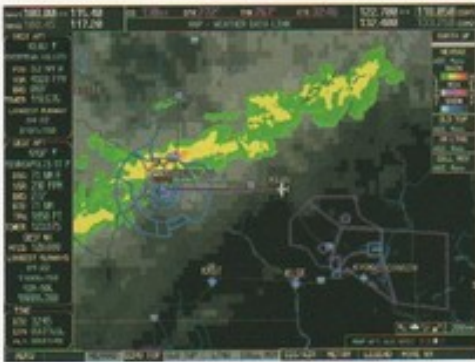
Weather datalink capability, via XM Satellite Radio and its XM WX Satellite Weather service, provides the G900X with color NEXRAD, METARs, TAFs, lightning, and other U.S. data displays.
