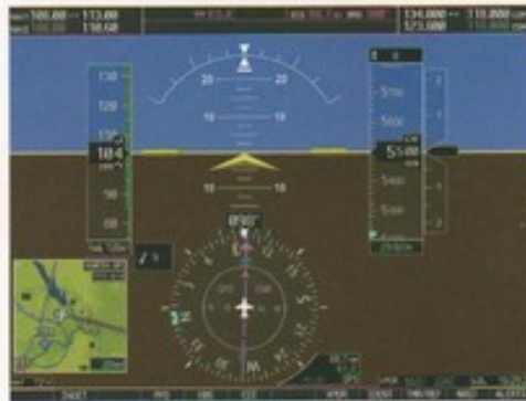
The plot's Primary Flight Display (or PFD) seamlessly integrates all situational information regarding the aircraft's position, speed, attitude, vertical rate, altitude, steering and flight progress.
