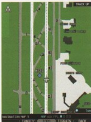
Helpful Garmin SafeTaxi™ airport diagrams identify runways, taxiways and hangars, as well as your aircraft location on field.
