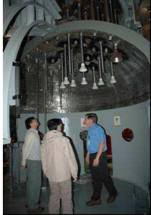
PWR 反應爐頂蓋 mockup 用以驗證 Control Rod Drive Mechanism (CRDM) 檢測技術
