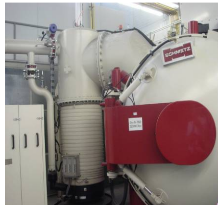
圖3-11 LVPS : 33mbar Preheat 700°C
