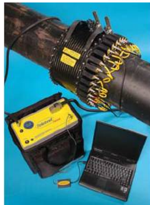
36" dia x 44mm thick gas compression station header inspected using Teletest® to detect corrosion at concrete supports
