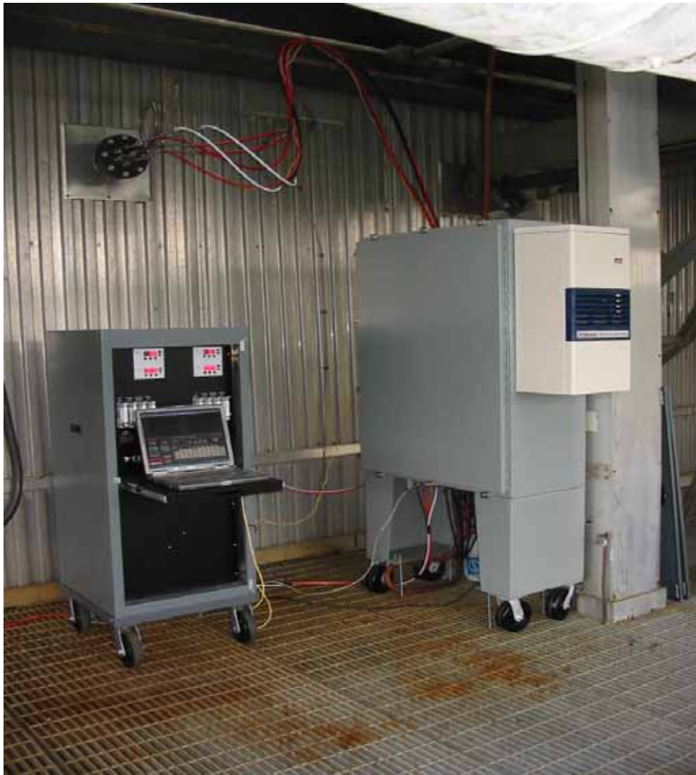
圖7. FERCo 的. In Situ Catalyst Activity Monitor, including:
