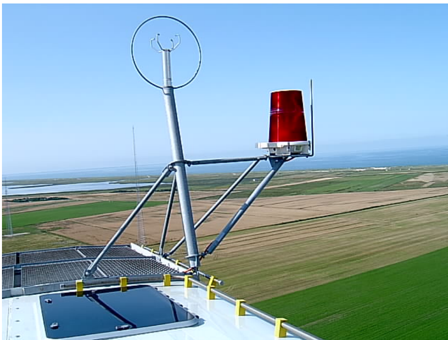
Figure 3 Ultrasonic anemometers and aviation lights on the rear end of the nacelle roof.
