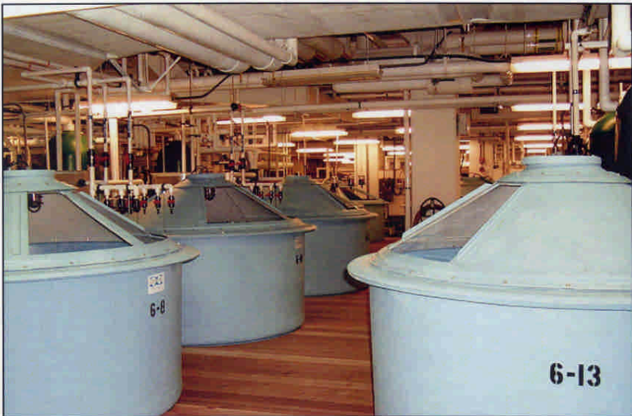
Recirculated fish tank with the biofilter (drum on the right) that uses beneficial microorganisms to remove the chemical waste from the water
