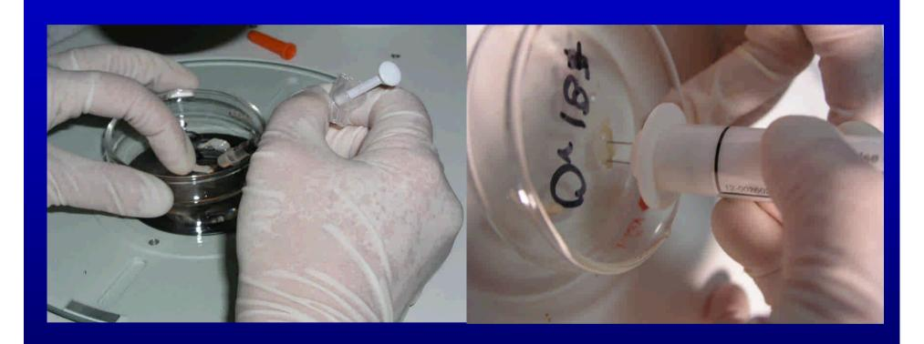
In situ Electorator (BTX); Voltage: 600-800 volts
