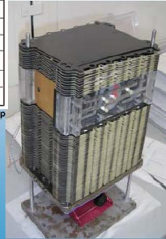
Assembly 1.3 kW DMFC Stack
