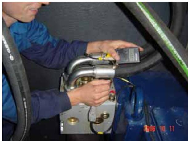
潤滑油 filter block 壓力檢查
