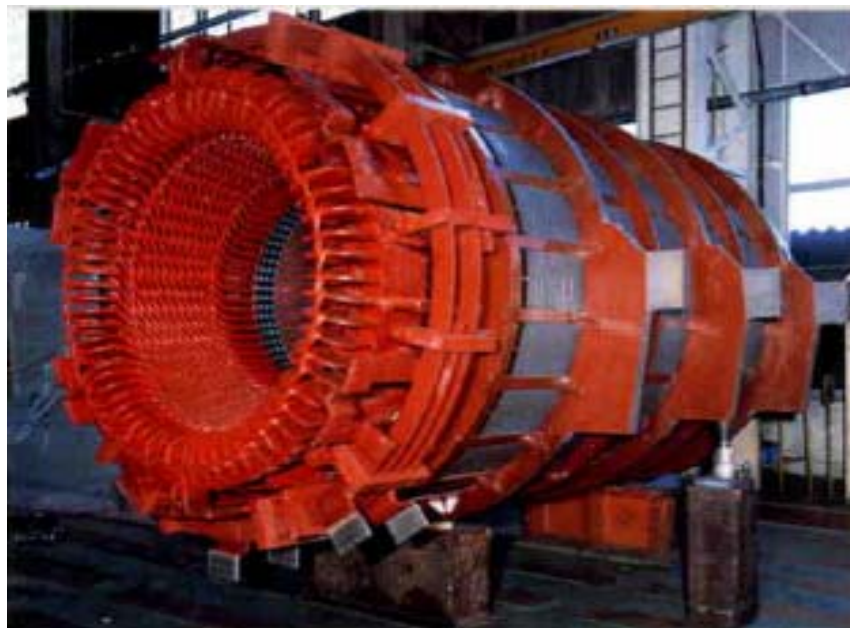
圖-11 Stator Assembly after Insulated with Global VPI Process (From Fuji Electric Systems Co., Ltd)
