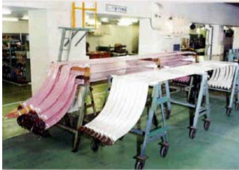
圖-10 Stator Conductors before Insert into Stator Core(From Fuji Electric Systems Co., Ltd)
