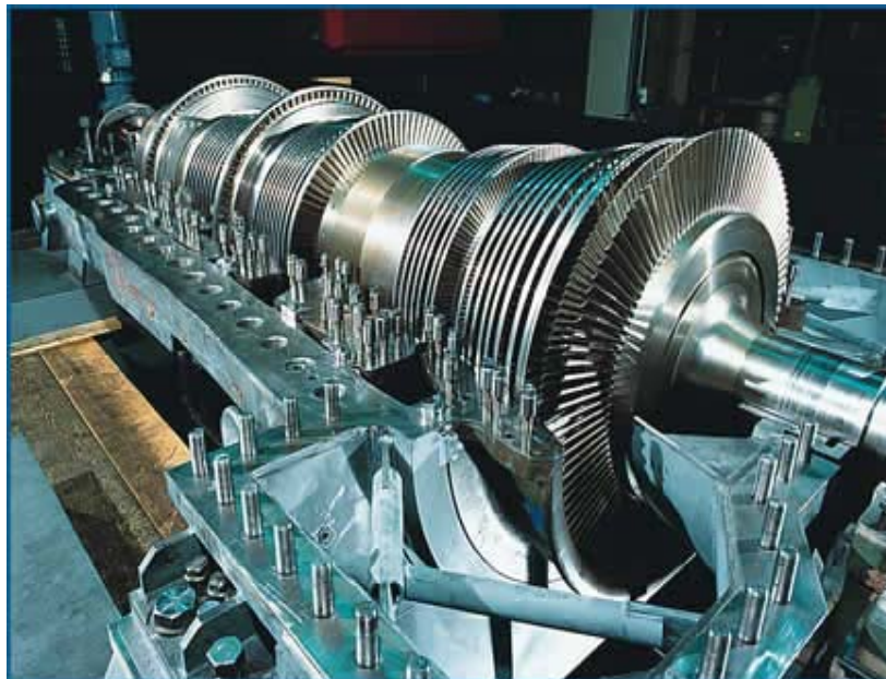
圖-7 CASING 組立(From Fuji Electric Systems Co., Ltd)
