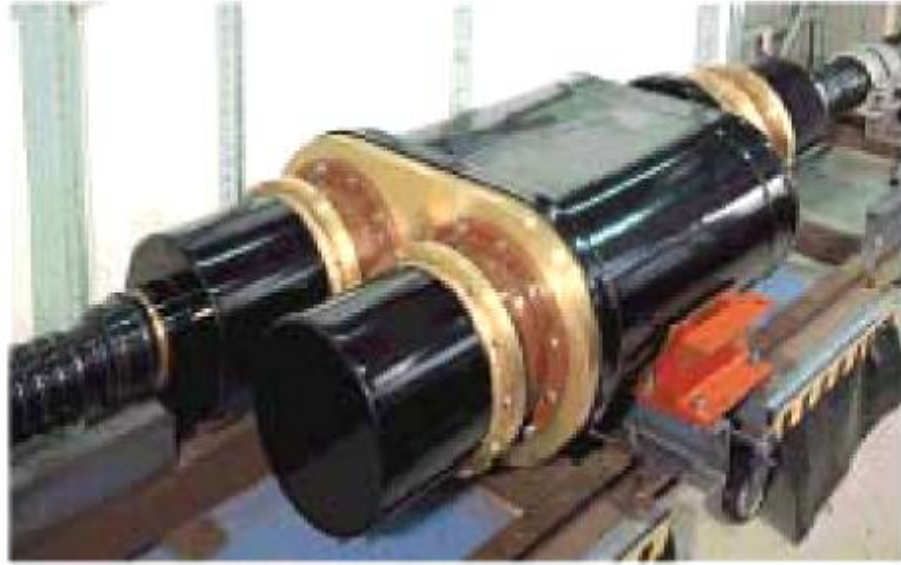
圖 3-13 Firstly adopted 275kV Y-branch Joint
