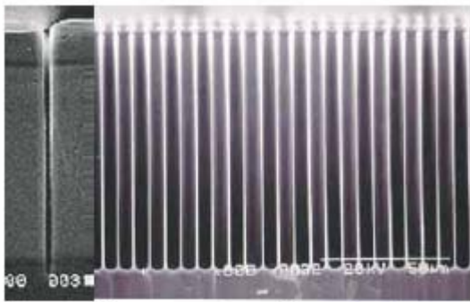
Fig. 3 High Aspect Ratio Etching using the A601E DRIE Etcher
