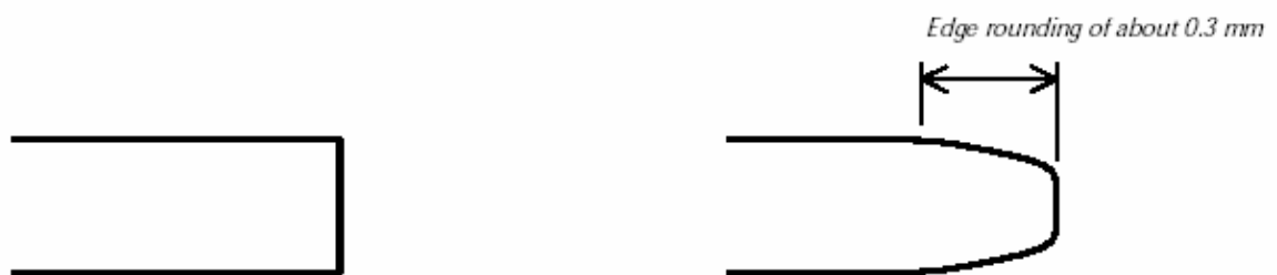
Wafer edge before and after grinding (front-end)
