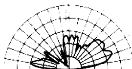
ELEV. DBE PATTERNS AT 100.0 DBE00 AZIMUTH AND FREQUENCY IS 30.000 MHZ MAX. GAIN IS 15.00
