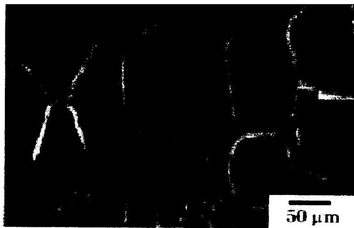
Foamed porous structure (PP) <SEM observation>
