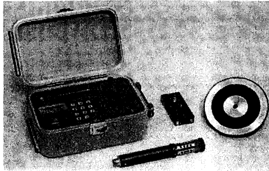
Fig. 2.1. Corrosion Rate Measuring Meter GECOR 6 [2,7]
