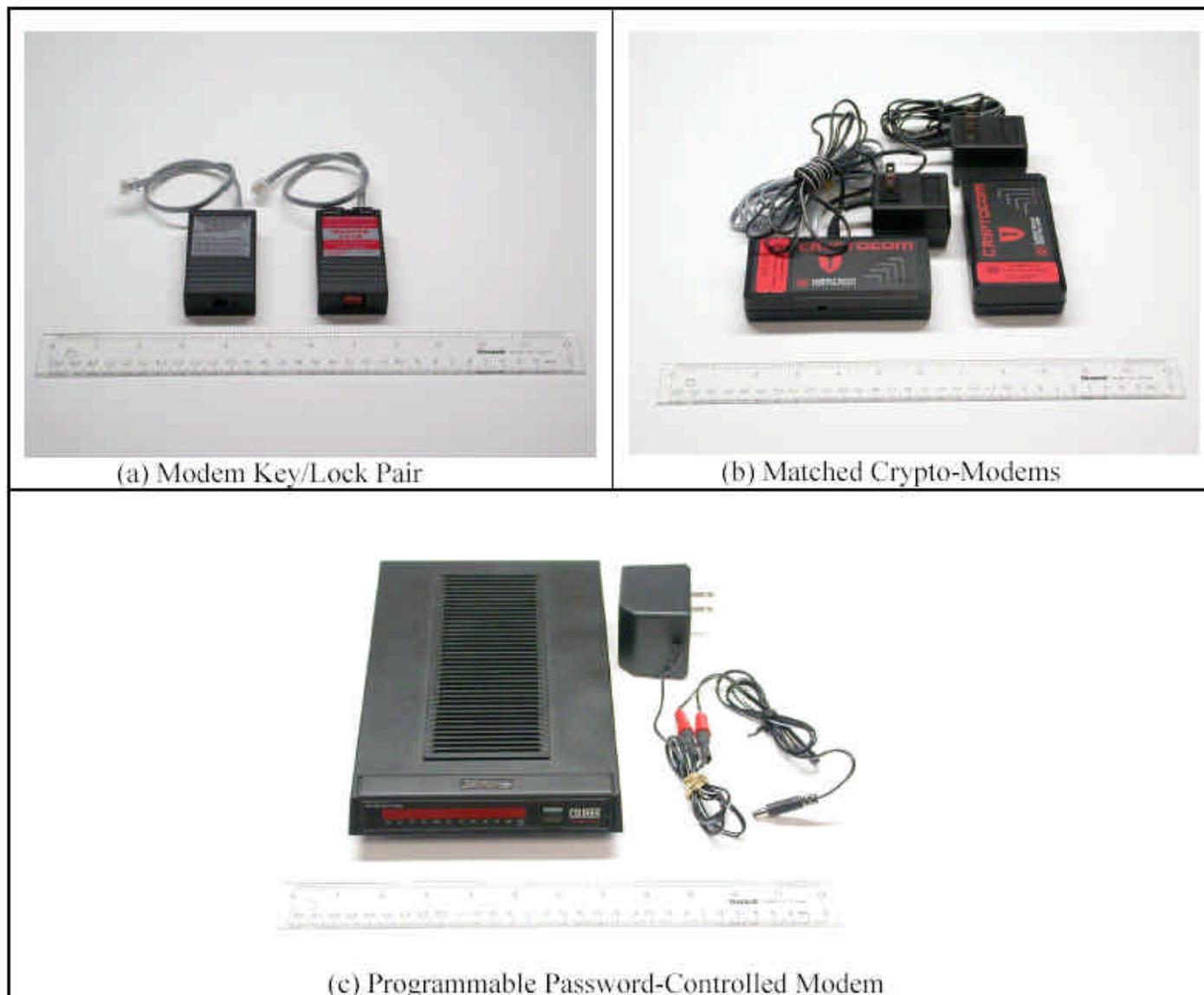
**Figure 7** Low-Cost Secure Modem Devices
