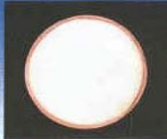
Pd penetration coupled with carrier interaction, pore characteristics and Pd crystallite size has strong effect on activity and selectivity.
