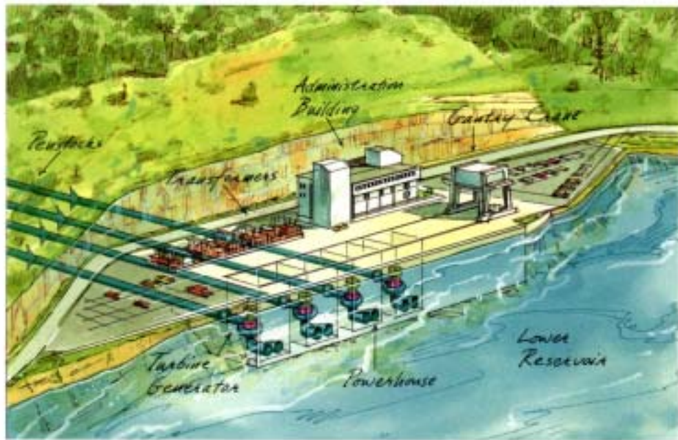
Artist's rendering shows water's journey through Brown Mountain. Each of the project's four turbine-generators can produce up to 260,000 kilowatts of electricity.
